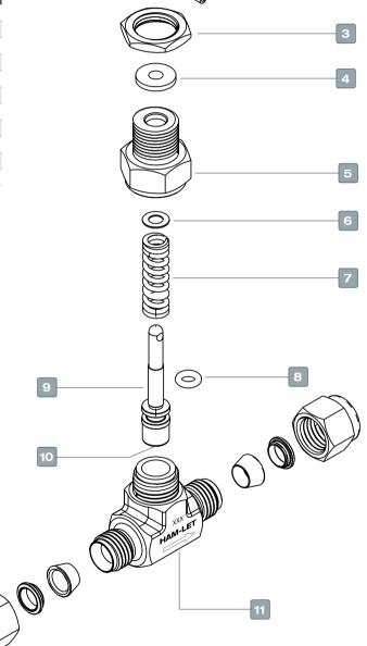
The H-1200 Series standard toggle valve is a compact design for normally closed and quick on/off service. Moving the handle 90 degrees upwards opens the valve to full flow and stops it firmly in the open position. Shifting the handle position downwards shuts off the valve by spring return. The PTFE soft seat at the tip of the stem provides a positive repetitive seal.
